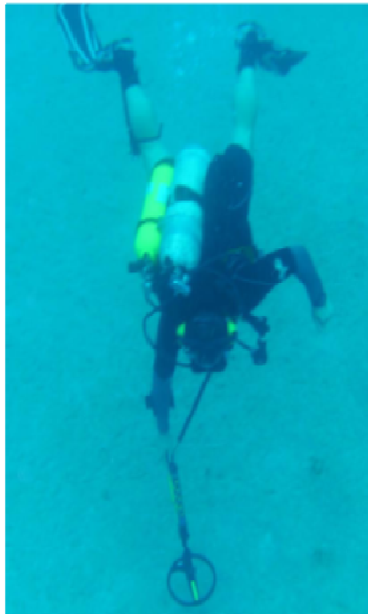
Figure 3-1: SCUBA UXO Divers using the Minilab Excalibur all metals detector
