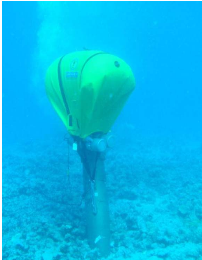
Figure 3-4: Mark V/ORCA-MOD 1 MVO 1000 Lifting Balloon with an 1100-pound lift capacity and Acoustic Actuation
